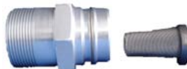
GTP-1534 Optional Strainer for all 1 1/2" actuators, except GTP-920-3S 24 x 110 mesh stainless steel. If you want the strainer and actuator assembly, order GTP-1510
